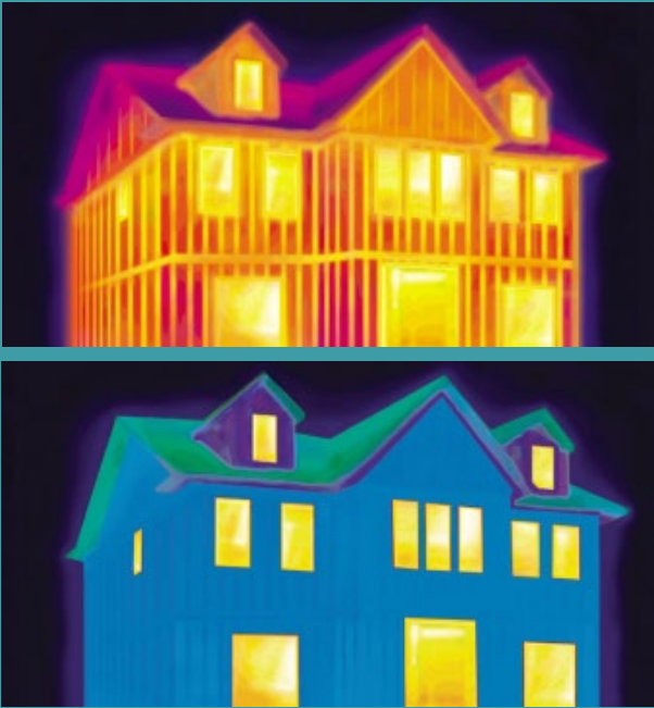
Figure 6: Example thermal images of a building demonstrating thermal bridges. Areas that are red and yellow show a lot of heat escaping through the building envelope. Blue and green areas show much less heat is escaping. Photo credit: Dow Chemical Company.
