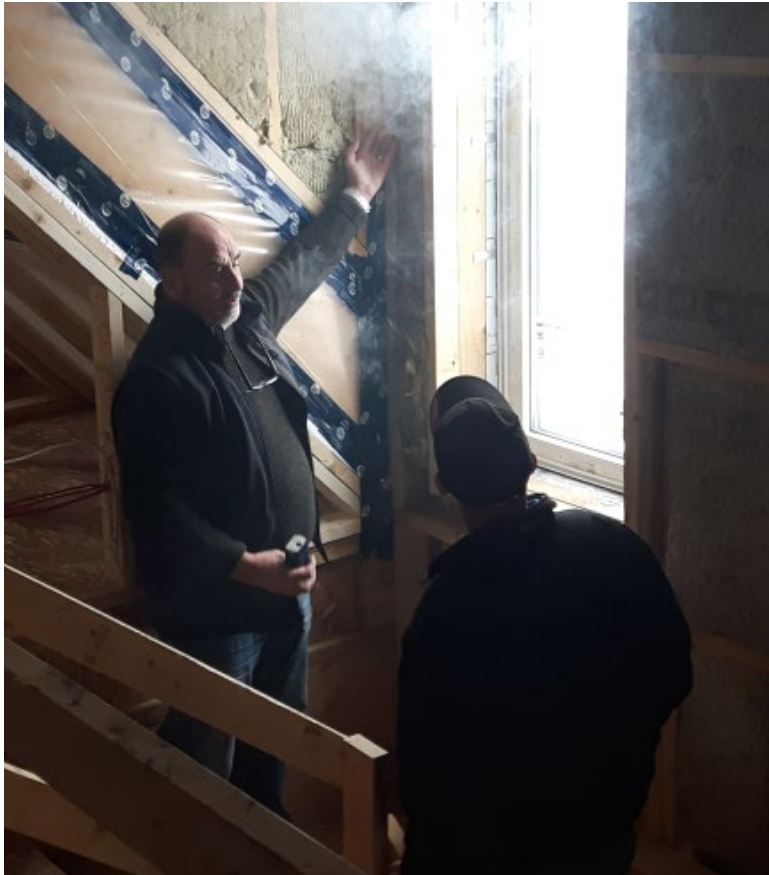
Right: Energy advisor Ray Smith shows a group of East Kootenay Regional District building officials how he uses a smoke machine to pinpoint leaks in a home's air barrier. Minutes previously, Smith depressurized the building with a powerful fan; the smoke reveals where outside air is rushing in to fill the vacuum via tiny gaps around the window.
