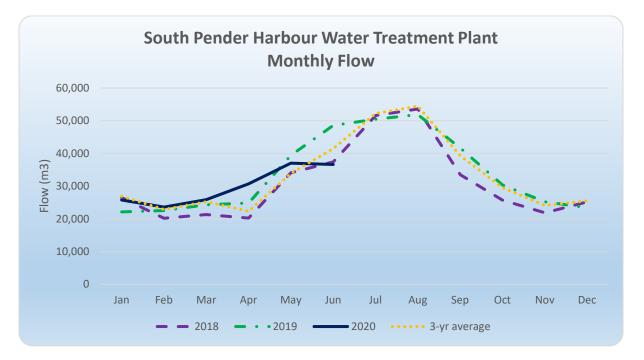
Note: The 2020 data is based on a new flow meter which is providing more accurate data than the meter used in 2018 and 2019
