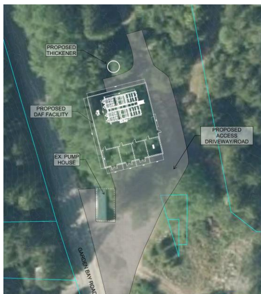
Figure 5-3. Proposed Building Footprint and Existing Garden Bay Water Treatment Plant
