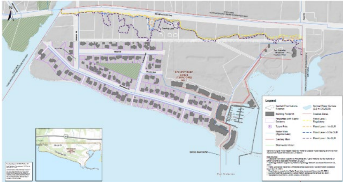
Figure 38: Flood hazard mapping for shisháhl Nation land No. 1, with up to 1m in sea level rise. Source: Kerr Wood Leidal, 2022.
