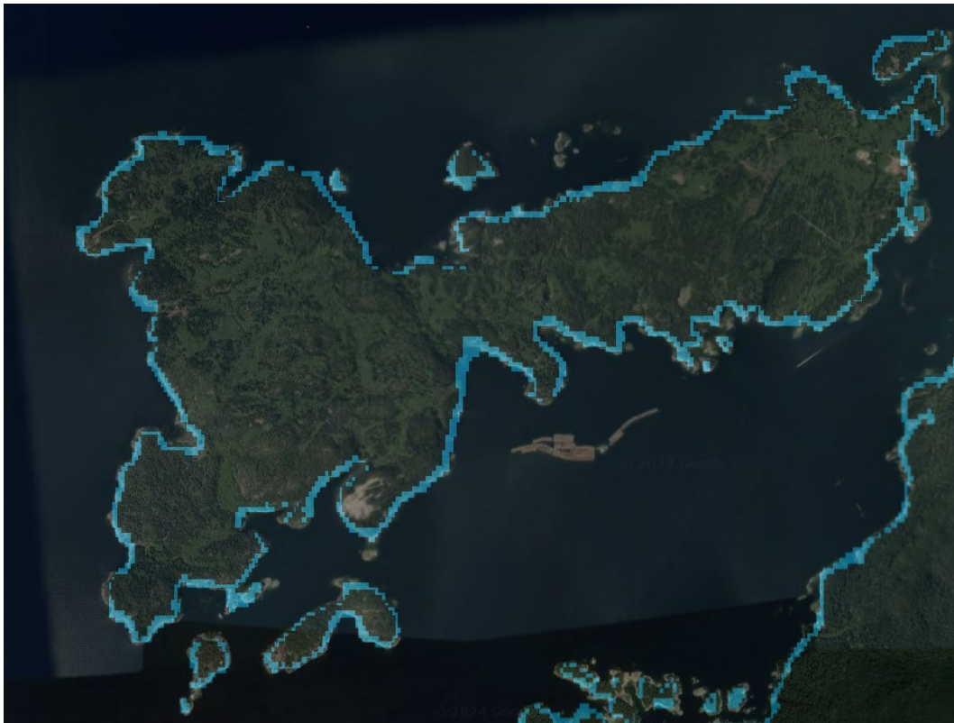
Figure 87: Hardy Island coastal flooding from sea level rise of 1m by 2100.
