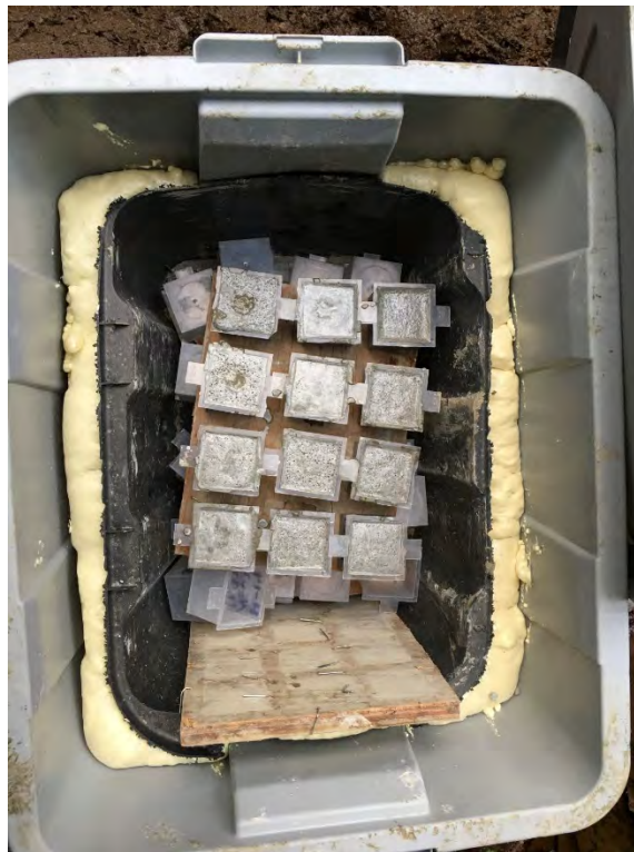
Photograph 2: Grout Samples Taken from the Grout Batch.
