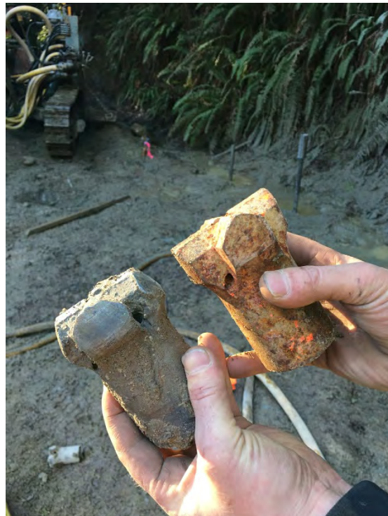
Photograph 4: Differences Between a Worn-Out Drill Bit (Left) and a New Drill Bit (Right).
