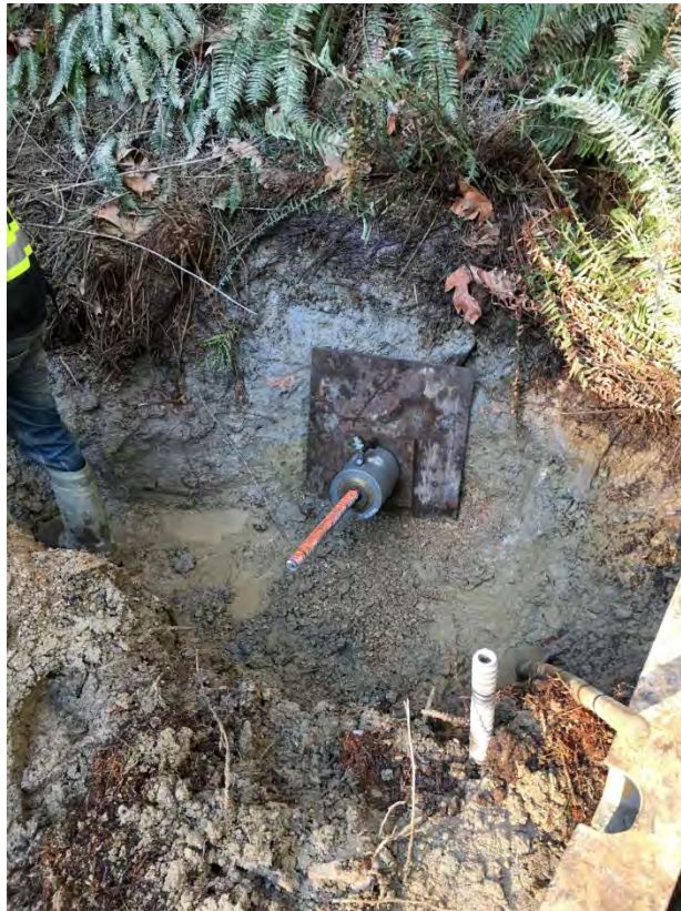
Figure 2: Prepared Test Pad at the End of Preparation
